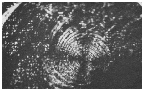
Figure 5 Spiral spherulite produced by acetone/chloroform treatment of spiral craze/crack system. Polarised light, polaroids crossed. Polycarbonate (×90).
